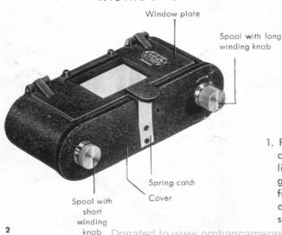
1. Press the spring catch on the cover, open the window plate, lift off the cover, and dust the glass plate and the printer. The following steps must be carried out in the darkroom by a red safelight.
